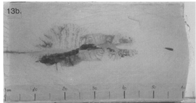
Fig. 8 M/94.3 in gelatin, range 2.5 m, v_i = 795-800 m/s
